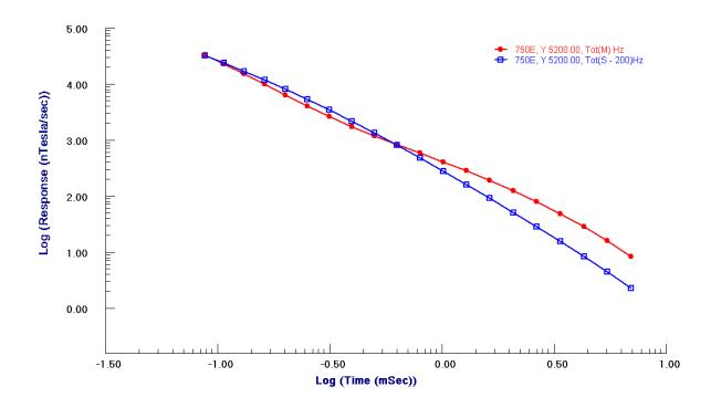
Plot measured data against model as a quick check. This simple half-space model does not fit the details of the decay but the amplitude is as expected. Proceed with further modeling, or inversion, as desired.
