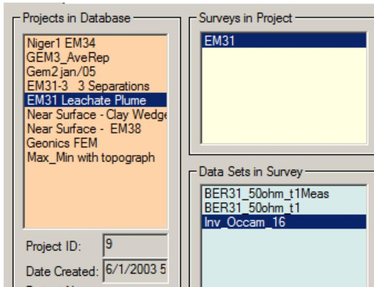
In each survey, there will be several data sets after modeling, inversion and processing. In this case, we have 1 forward model and 1 inversion model. The forward model has a new data set containing the simulated data under the model. Similarly, each inversion contains a new dataset containing the simulated data set under the inversion model (for each point) and attached to that data set is the inversion model.
