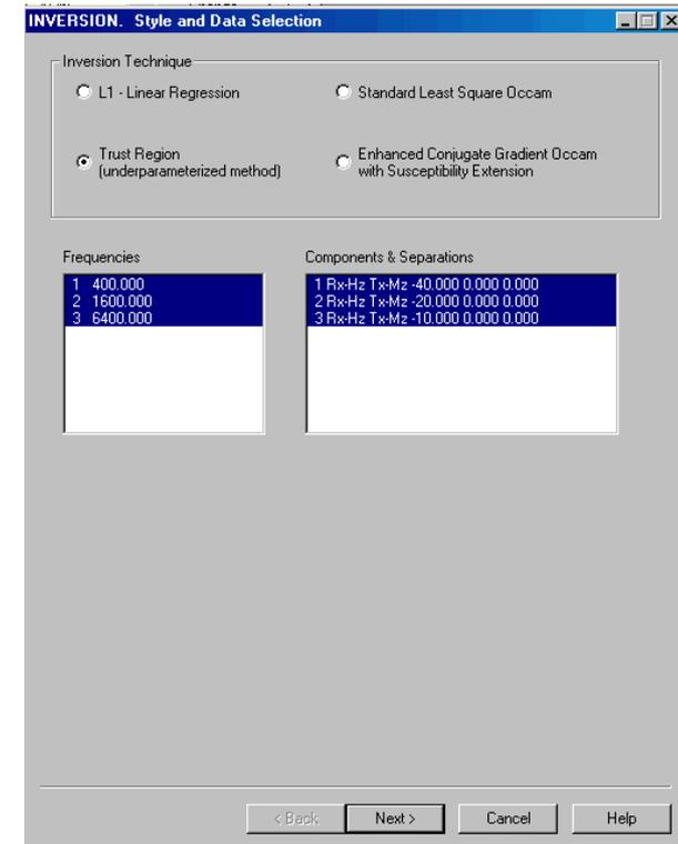
In this case, we will be utilizing a 3 frequency EM34 dataset, with 3 separations each at its own frequency.
