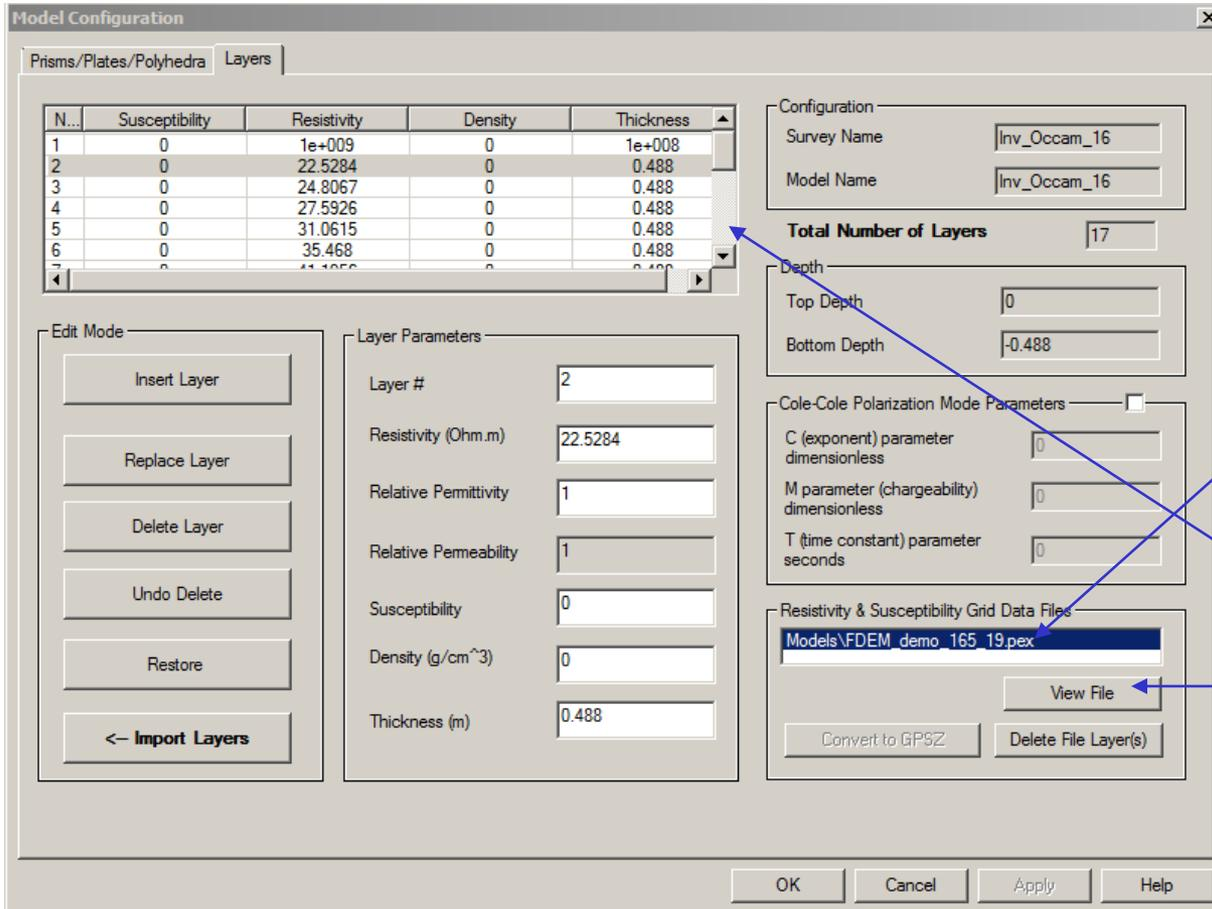
Attached to the database in a subdirectory called “Models” is the inversion results in a simple ASCII XYZ file (\*.pex) which may be viewed here. This file may easily be imported to another application although graphical viewing tools are provided within EMIGMA.
