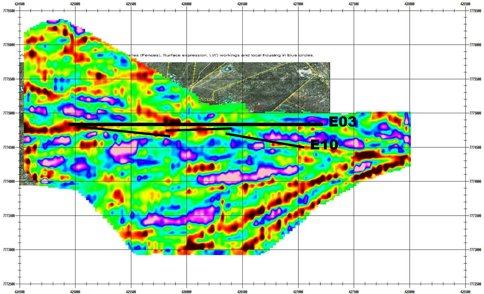
**Figure 23: 1999 UTS Mag Data, Reduced to Pole, Vertical Derivative with Tops of EM Structures**
