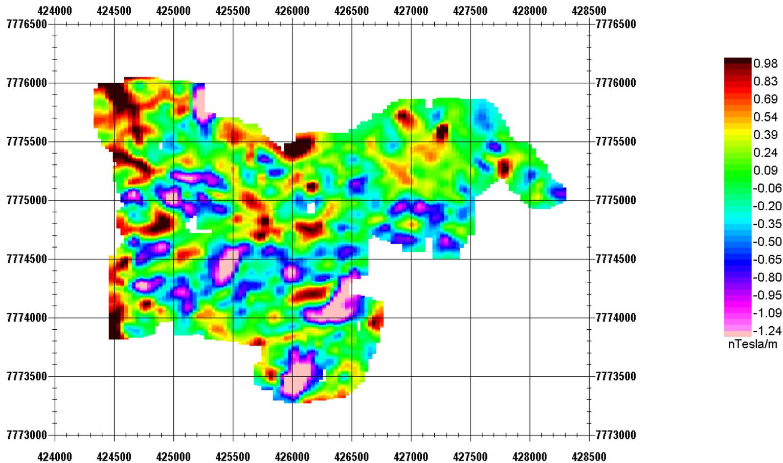
**Figure 13: 2008/2010 Ground Data – Upward Continued to 50 m, Vertical Derivative**
