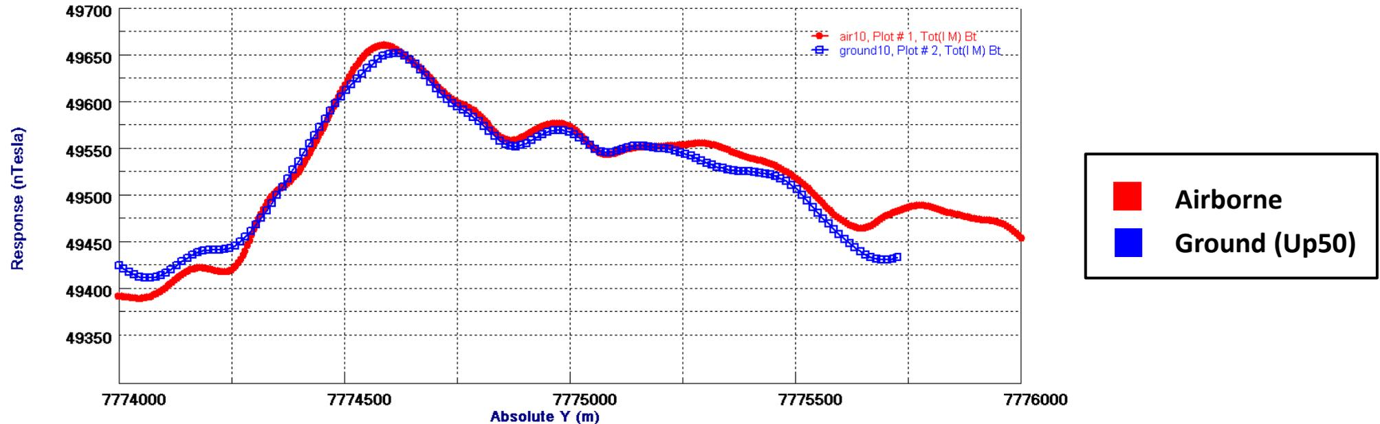
**Figure 15: Profile response comparisons of upward continued ground data to airborne data**
