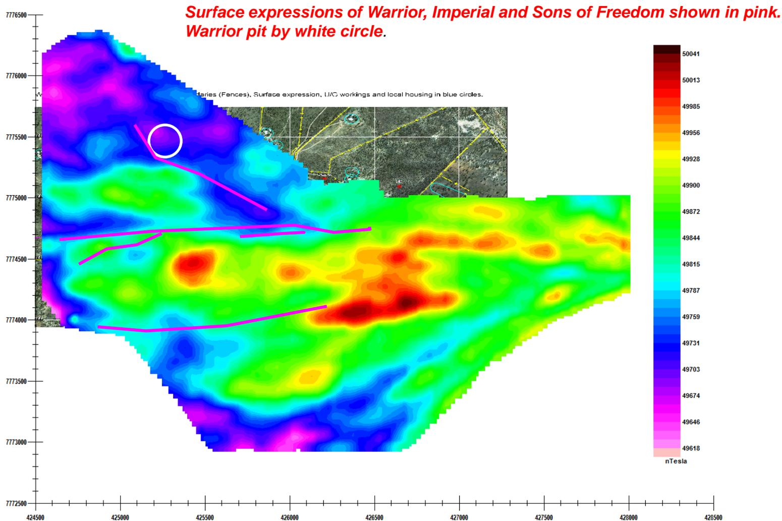
**Figure 18: 1999 UTS AeroMag Data, Reduced to Pole, Total Field**
