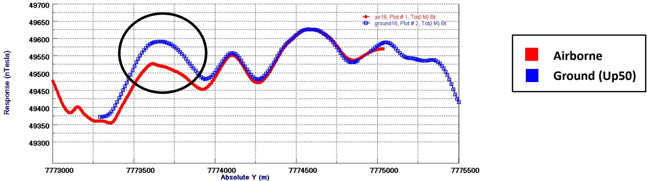
**Figure 16: Profile response comparisons of upward continued ground data to airborne data**
