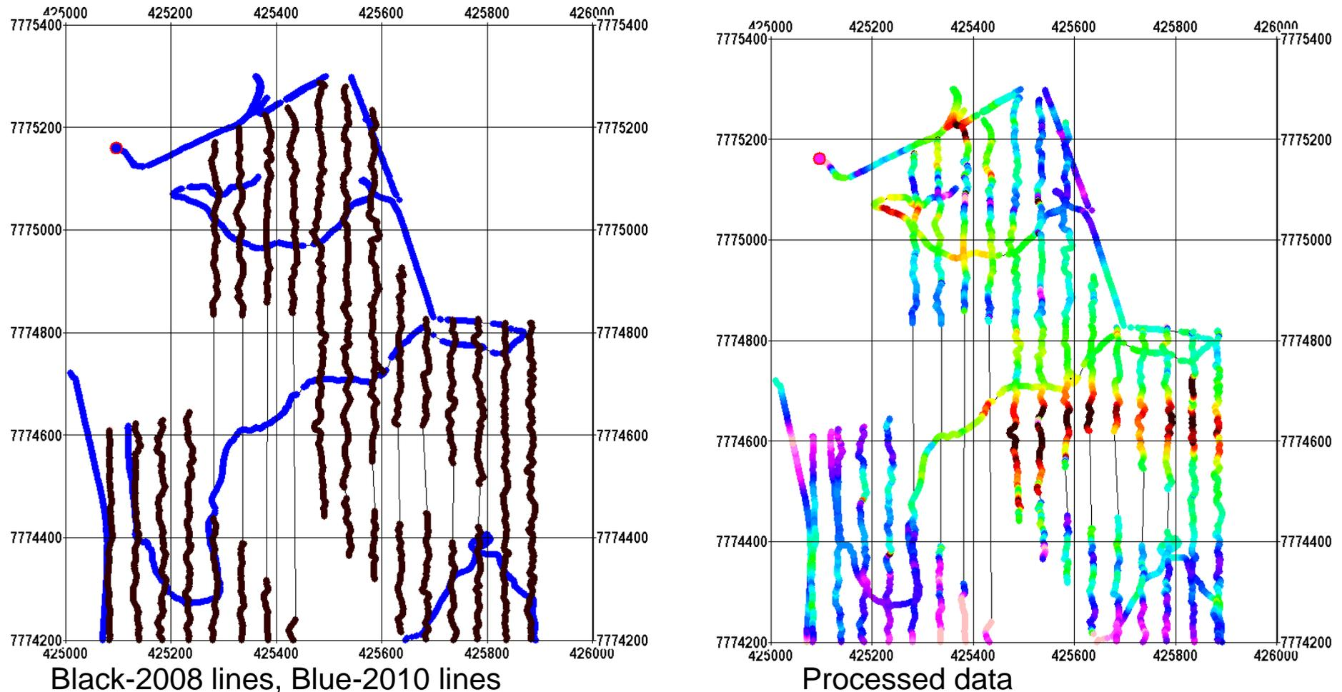
The 2010 data was shifted to the level of the 2008 data as the final step in the processing. The data was later compared at intersections and nearby lines in two areas to check for agreement: 1) Northwest and 2) South.
