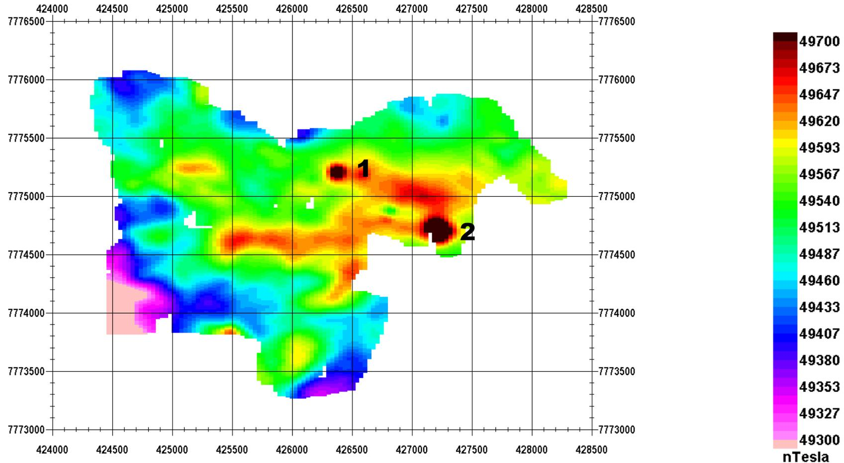
**Figure 9: 2008/2010 Ground Data – Upward Continued to 50 m**
