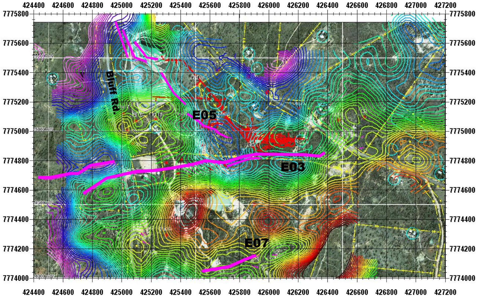
**Figure 12: 2008/2010 Ground Data – Upward Continued to 50 m, RTP – REPROCESSED, Close-up with satellite underlay. E03, E05 and E07 structures are shown in pink.**
