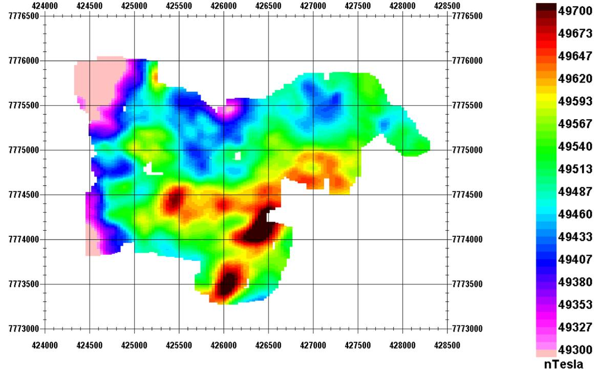
**Figure 11 2008/2010 Ground Data – Upward Continued to 50 m, RTP – REPROCESSED**
