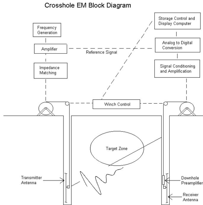
**Figure 5: System components and standard survey setup.**
